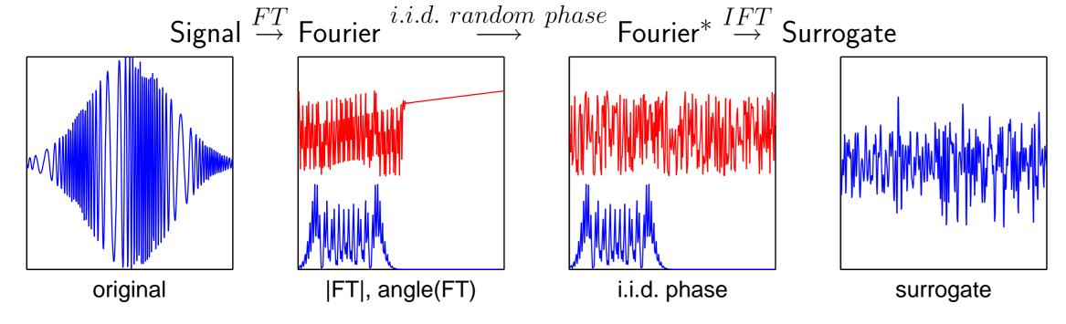
Use of Surrogates for Non-linearity tests. — The Non-linearity test is applied to a set of surrogates.
